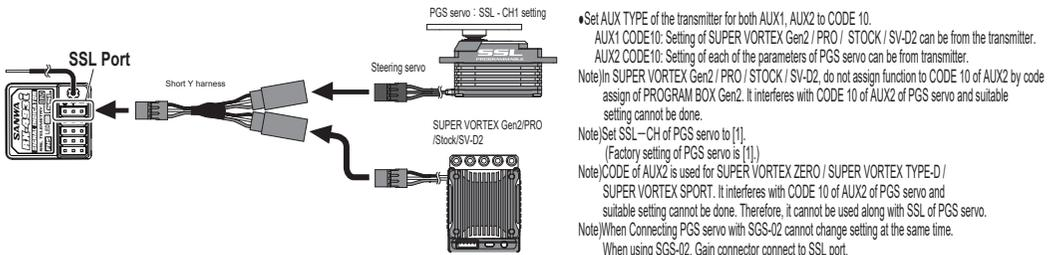
●Set AUX TYPE of the transmitter for both AUX1, AUX2 to CODE 10.
