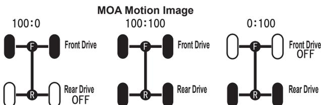
\*By changing the ratio, you can adjust the gear ratio of front-rear.
