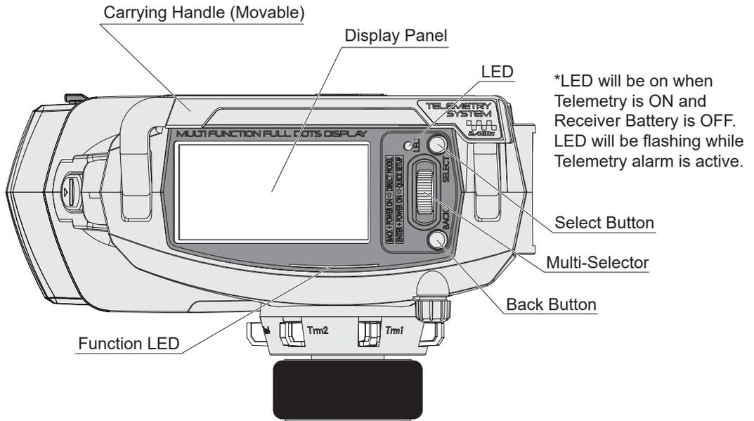
\*LED will be on when Telemetry is ON and Receiver Battery is OFF. LED will be flashing while Telemetry alarm is active.
