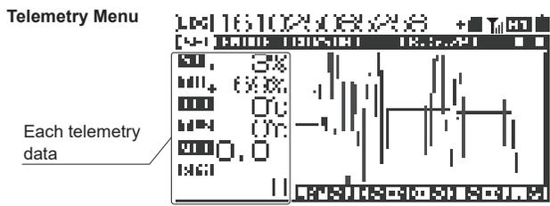
When using RX-491/492/493/493i and SUPER VORTEX Series/PGS Servo Series/SGS-02, Turn telemetry function on, then display telemetry data from receiver.
