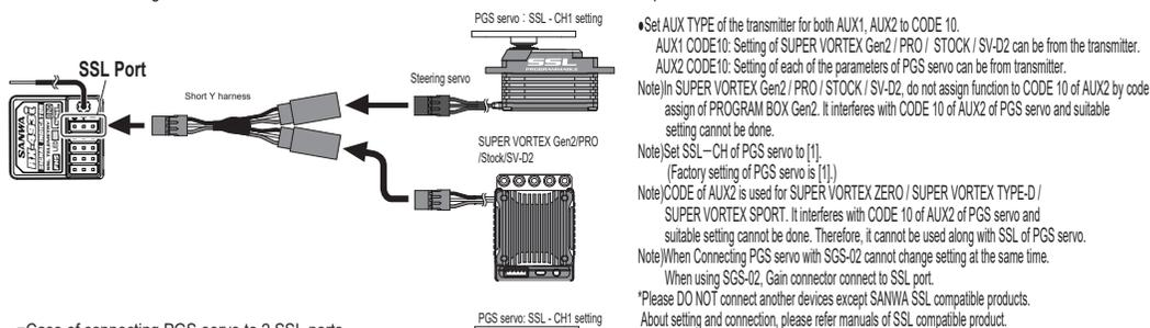
■Case of connecting PGS servo to 2 SSL ports
